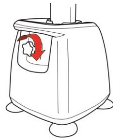
Figure 2-3: Clamping handle tightening
