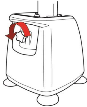
Figure 4-1: Clamping handle loosening
