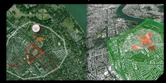
A top-down 2D perspective is the most commonly used visualization technique in drone detection. The 3D view expands our capabilities by adding the drone's altitude information (this requires multiple drone detection systems), and making it easier to evaluate distances between different objects on the map.
